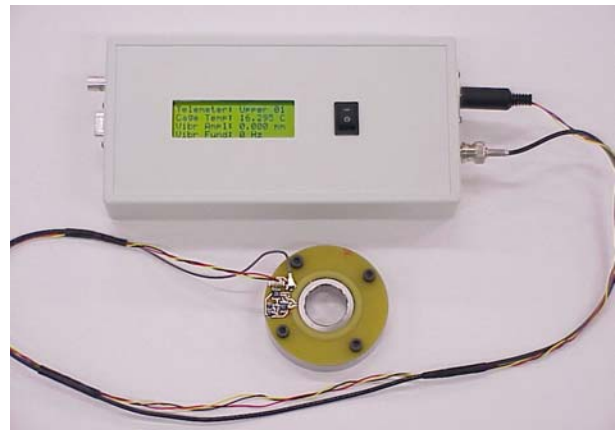
Figure 6. Instrumented bearing with cage transponder, excitation/measurement circuit, and signal processing unit.
