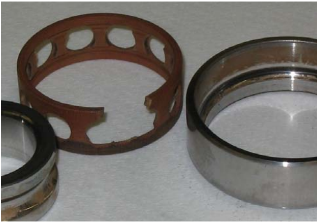
Figure 4. Failed ACW bearing cage from lubricant starvation test. Note dust on races from cage wear.
