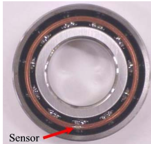
Figure 5. ACW angular contact bearing with transponder installed in cage.
