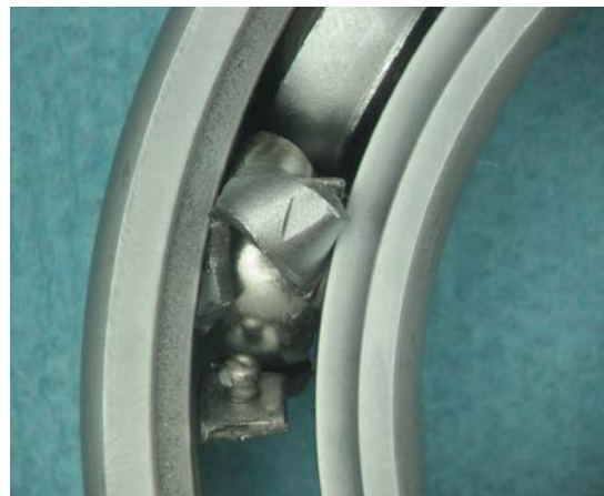
Figure 3. Failed UH-60 hanger bearing from lubricant starvation test.
